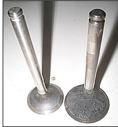
Illustration 1 On the left is my brand new 36mm exhaust valve. On the right is a very coked up inlet valve, from my scrap head
